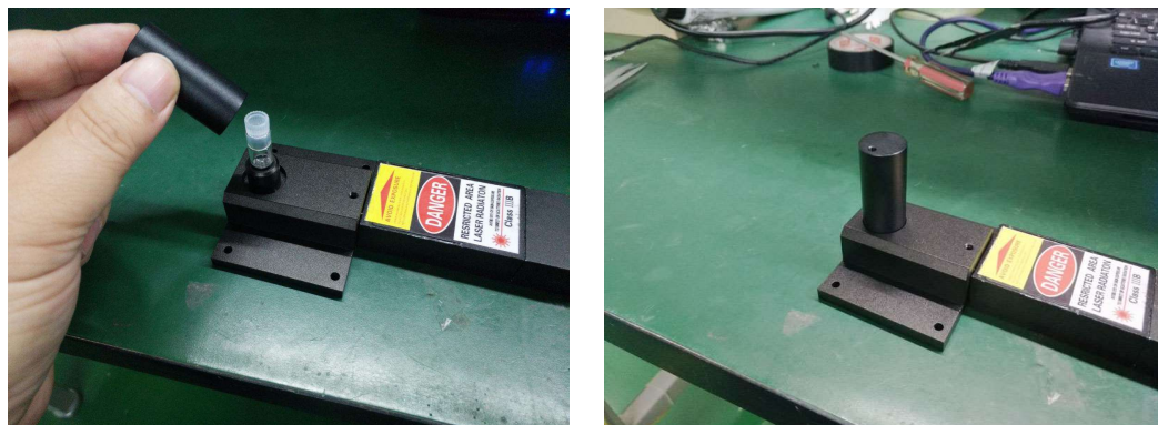
Fig 2 Fluid sample cell (Liquid chromatography bottle) (Optional)
