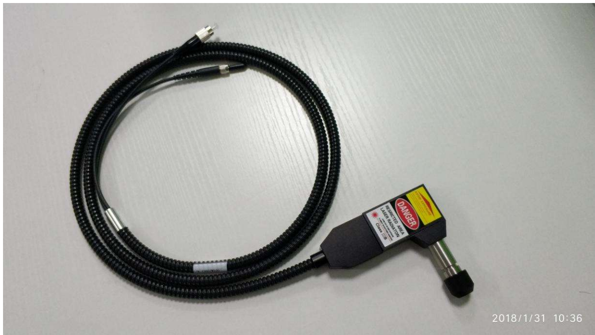
Fig 5 Raman probe gun (optional)
